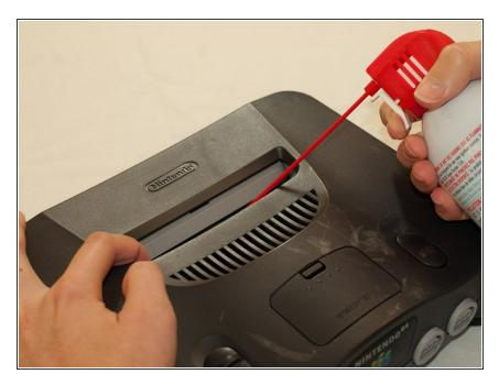
Open the slot with your finger. Blow along the length of the cartridge slot with the air duster.
