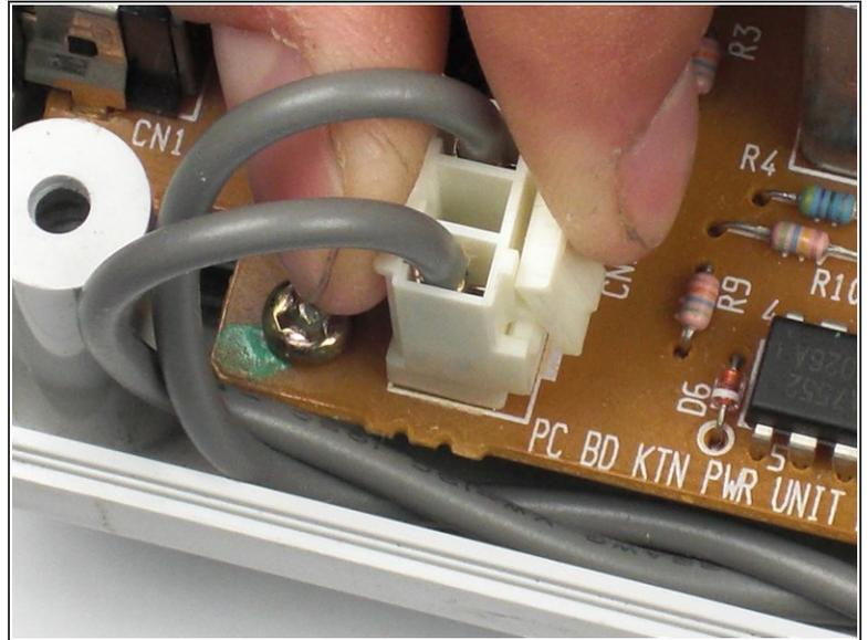
**⚠** Verify that the console is disconnected from the AC outlet before you begin. If you have just powered off the system, give the capacitors a few minutes to discharge before you begin working.
