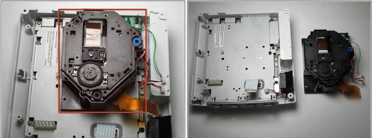
**!** When lifting the GD-ROM, be careful that the top half of the casing does not detached from its base.
