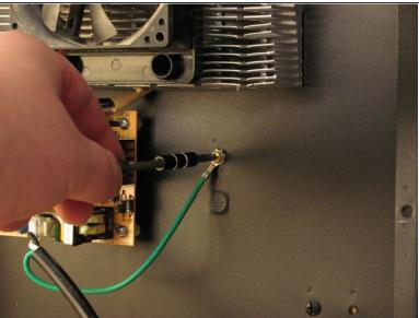
Remove one 12mm Phillips screw securing ground.
