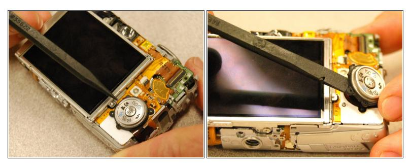
Identify and remove the plastic function set button. Do this by gently prying up as indicated in the photo.
