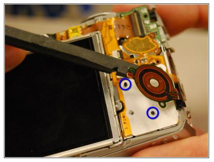
• Lift the function set button ribbon cable from the two guide pins.
