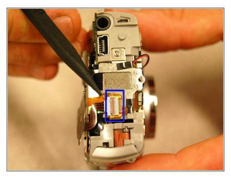
• Remove the ribbon cable by lifting on the flat tab and pulling the ribbon cable from the connection.
