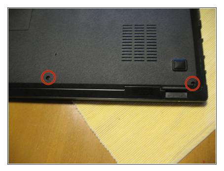
Remove the two 5mm screws near the front of the computer
