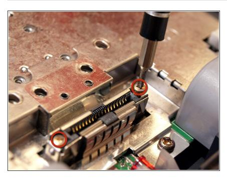
Remove the two screws indicated in the example using the smaller Phillips screwdriver.
