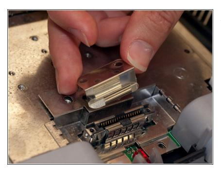
Remove the small metal bracket from the back of the expansion pack slot.
