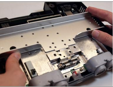
Remove the metal plate indicated in the example by sliding it back and then lifting it up.
