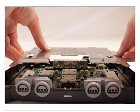
Lift off and remove the metal plate as indicated in the example.
