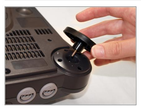
Remove the two front feet of the N64.
