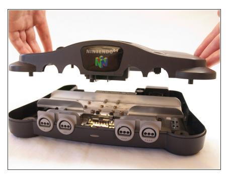
Rotate to top side up and lift off top cover.
