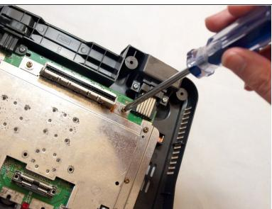
Remove the seven screws indicated in the example using the larger Phillips screwdriver.
