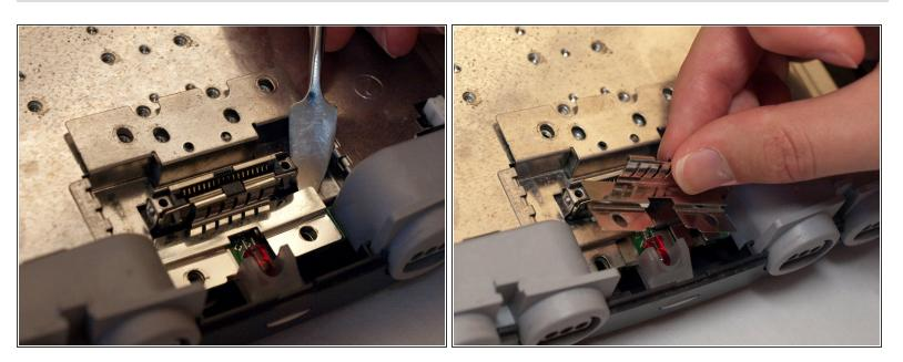
Remove the small metal bracket from the front of the expansion pack slot with the metal spudger.
