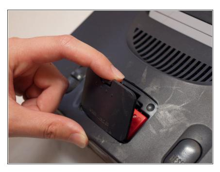
Remove the expansion pack cover by pushing in the tab and pulling out.
