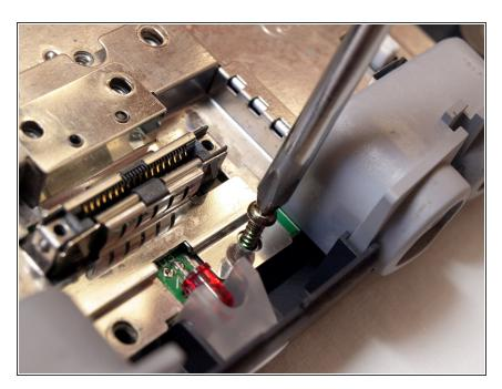
Remove the screw to the right of the LED light using the larger Phillips screwdriver.
