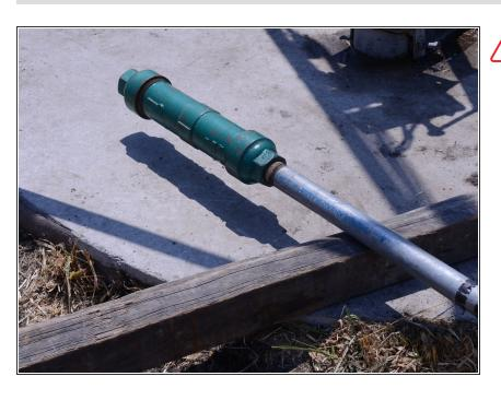
Make sure to keep the cylinder off the ground to prevent contamination.
