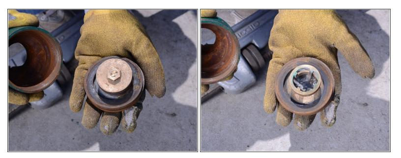
Check the foot valve components for signs of wear.
