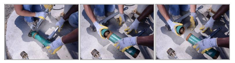
Using two pipe wrenches, remove the end cap from the cylinder.
