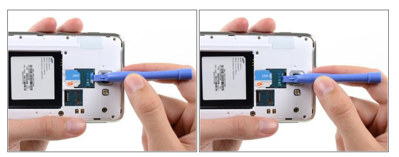
• Use a plastic opening tool, or your fingernail, to push the SIM card out of its compartment.
