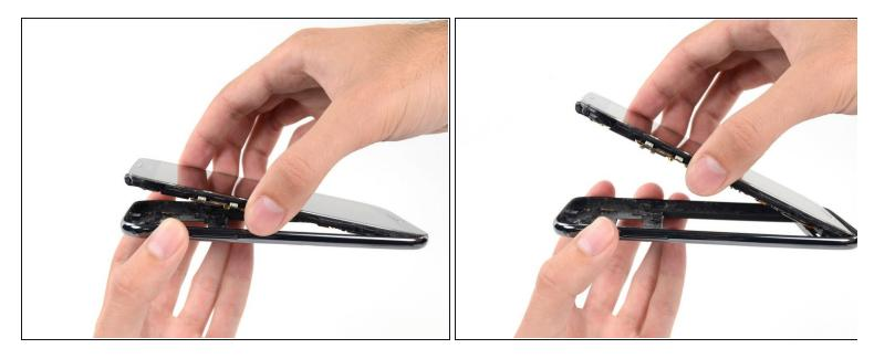
• Lift the display assembly out of the midframe.
