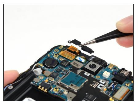
• Remove the front-facing camera bracket.
