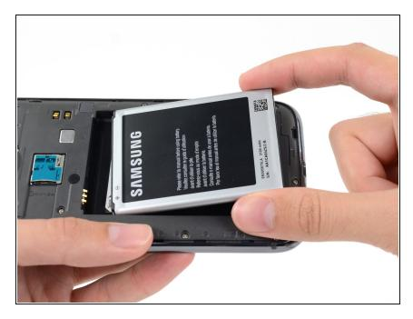
• Remove the battery from the midframe.
