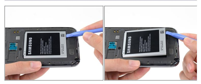
Insert a plastic opening tool, or your finger, into the notch of the battery compartment and lift the battery upward.
