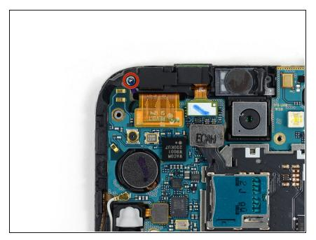
Remove the 3mm Phillips #00 screw from the front-facing camera bracket.
