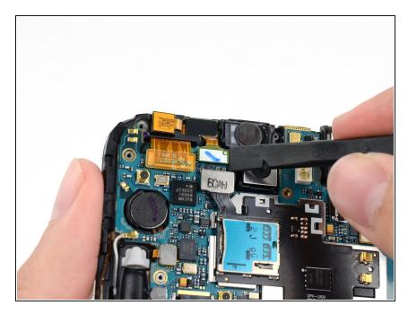
• Use the flat end of a spudger to disconnect the front-facing camera connector.
