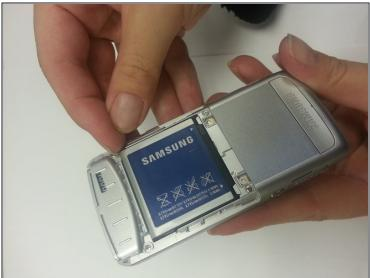
• Using your finger, grasp the corner on either side of the battery and pull up.
