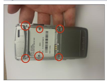
Unscrew the four corner .4cm Phillips head screws and the two middle .3 cm Phillips head screws.
