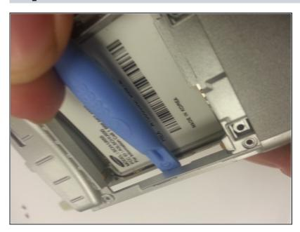
Gently insert the plastic opening tool into the seam where the battery was located.
