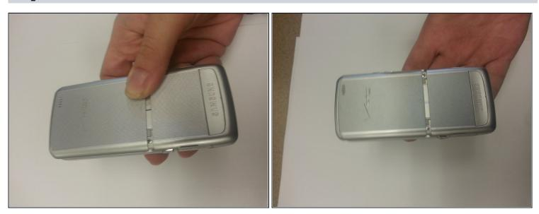
• Using your thumb(s) slide the battery cover up to remove it.
