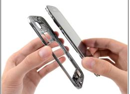
Remove the midframe from the display assembly.
