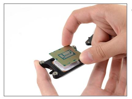
• Remove the CPU from the heat sink. Be careful not to touch the contacts.
