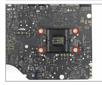
• Remove the four 12 mm T10 shoulder screws from the spring plate behind the CPU.
