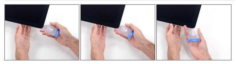
• Insert a second plastic card into the gap between the display and frame located at the top left corner of the iMac.
