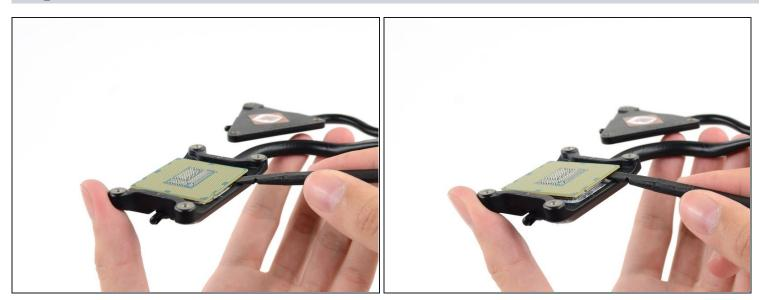
(*i*) The CPU will most likely be stuck to the heat sink with thermal compound.
