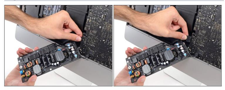
Be very careful not to touch the capacitor leads or any exposed solder joints on the back of the power supply. Only handle the board by the edges.
