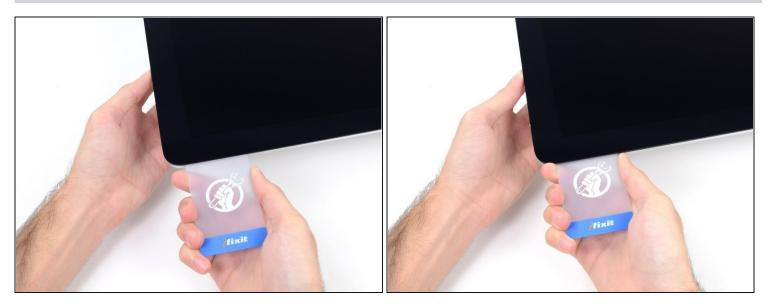
• Wedge the plastic card into the top right corner once again and let it stay there to keep the adhesive from resettling.
