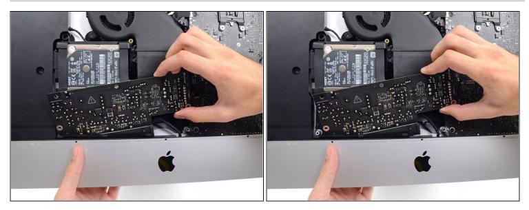
• Slide the power supply to the right to clear the screw posts on the rear enclosure.
