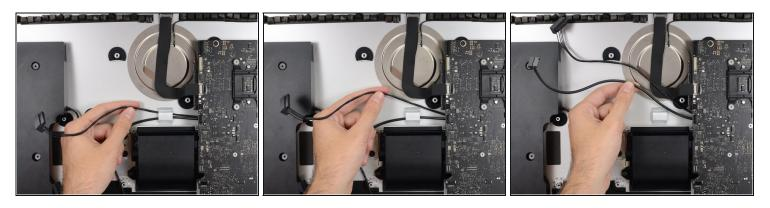
• In a similar fashion as the previous step, de-route the SATA data and power cables up out of the retaining clip.
