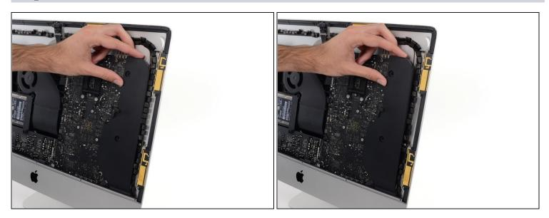
• Pull the top of the right speaker away from the rear enclosure, about half an inch, to expose the antenna cable running down its right side.
