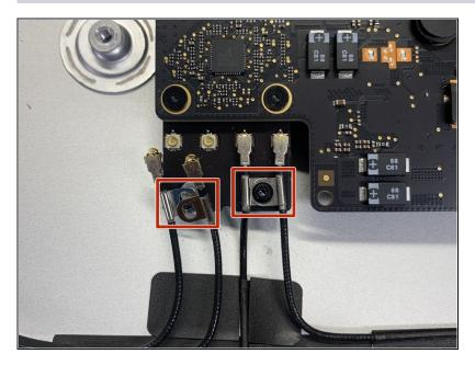
• If brackets secure the four antenna cables, remove the two T5 Torx screws from the brackets.
