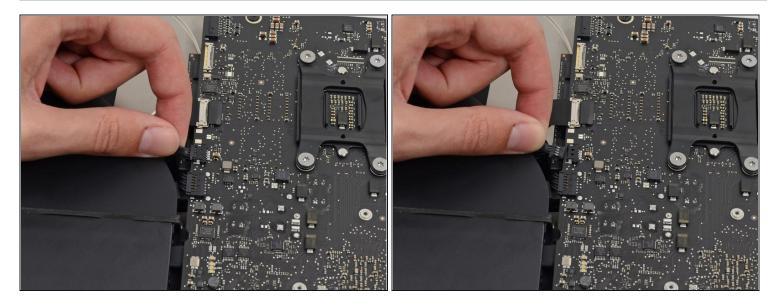
• Gently pull the fan cable connector straight away from its socket on the logic board.
