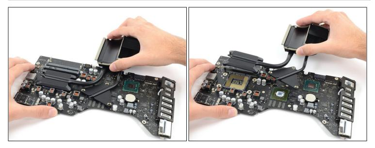
• Lift and remove the heat sink up off the logic board.
