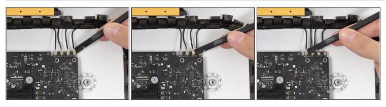
• Use the flat edge of a spudger to disconnect each of the four antenna connectors from the AirPort/Bluetooth card.
