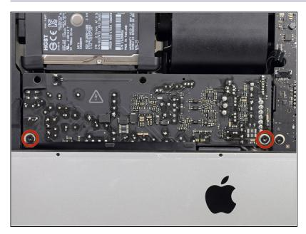
Remove the two 7.2 mm T10 screws securing the power supply to the rear enclosure.
