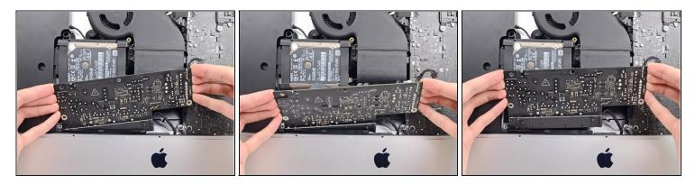
• Rock the power supply forward and remove it from its recess in the rear enclosure.
