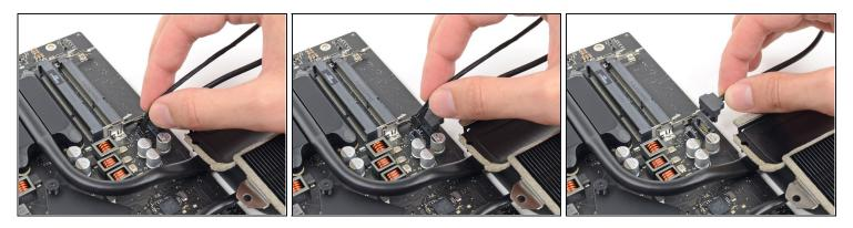
• Disconnect and remove the SATA data and power cables from the logic board.
