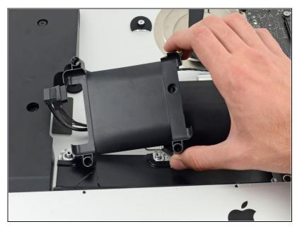
• Remove the hard drive tray from the rear enclosure.
