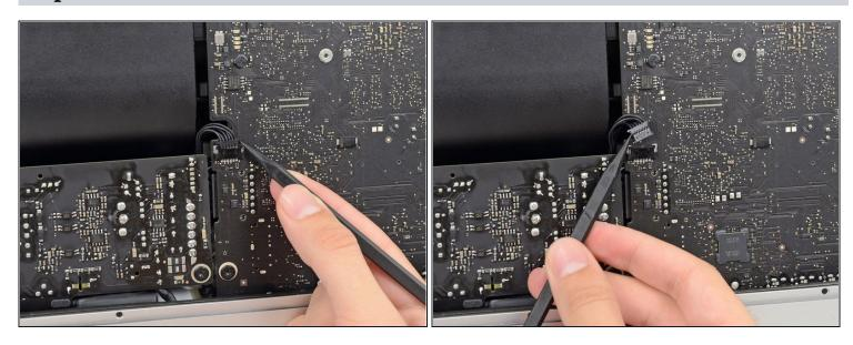
• Gently push upward on each side of the power supply control cable connector with the tip of a spudger to gently "walk" it out of its socket.
