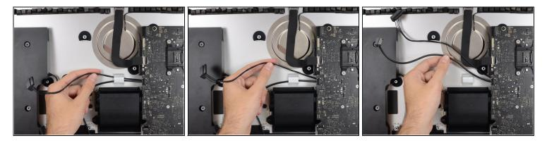
• In a similar fashion as the previous step, de-route the SATA data and power cables up out of the retaining clip.
