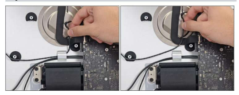
• De-route the left speaker cable by pulling it straight up out of the retaining clip in the back of the rear enclosure.
