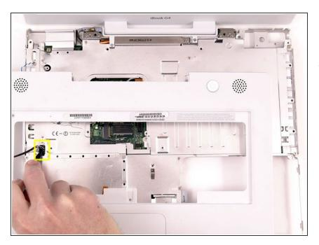
Carefully disconnect the multicolored speaker cable from the logic board. As before, make sure you're pulling only on the connector and not on the socket.
