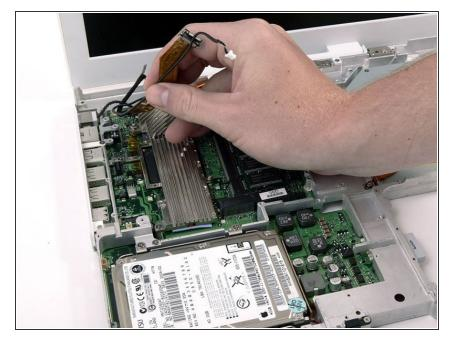
Deroute the microphone and display data cables from the metal framework, removing tape as necessary.
