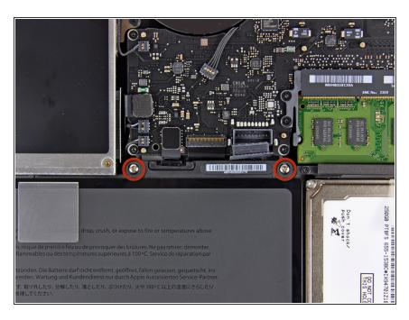
Remove two 5 mm Tri-point screws securing the battery to the upper case.
