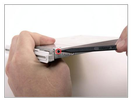
Hold the optical drive on its side and depress the remaining tab to free the bezel from the drive.
