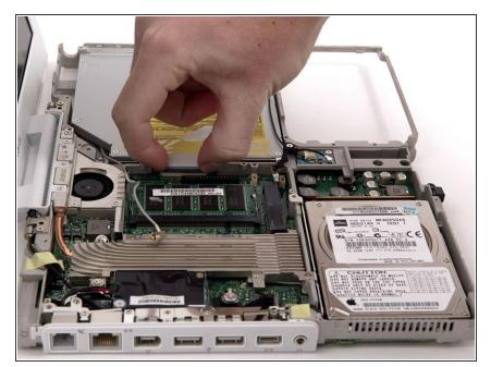
Release the optical drive ribbon clamp as described above. Slide the optical drive ribbon out of its connector.
