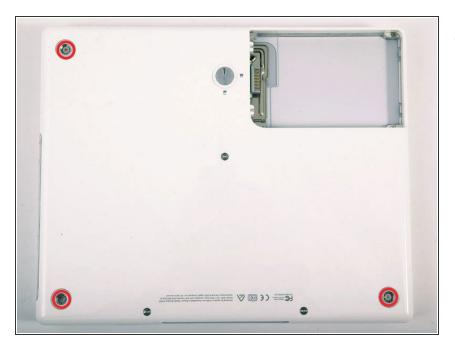
Remove the three newly-revealed Phillips screws.
