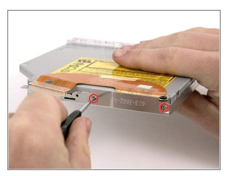
Remove the two Phillips screws securing the metal bracket and cable to the back of the optical drive.
