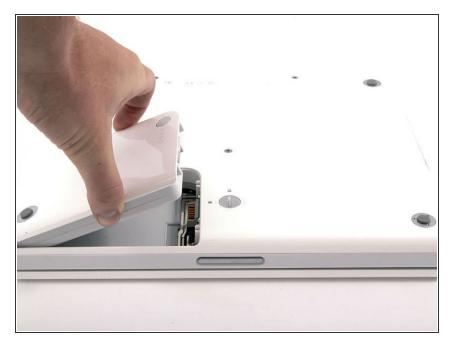
Lift the battery out of the computer.
