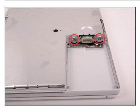
Remove the small greasy springs with white plastic caps from either side of the battery contacts.
