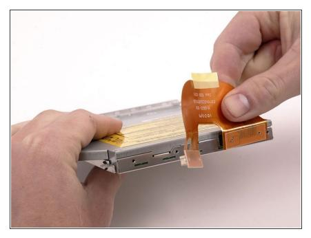
Peel the orange cable up from the top of the optical drive, removing tape as necessary, and disconnect it.
