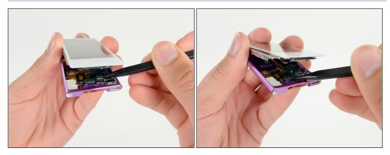
• Use a spudger to release the digitizer cable and display data cable connectors.
