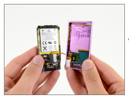
• Gently unfold the two halves of the device to access the internal components.
