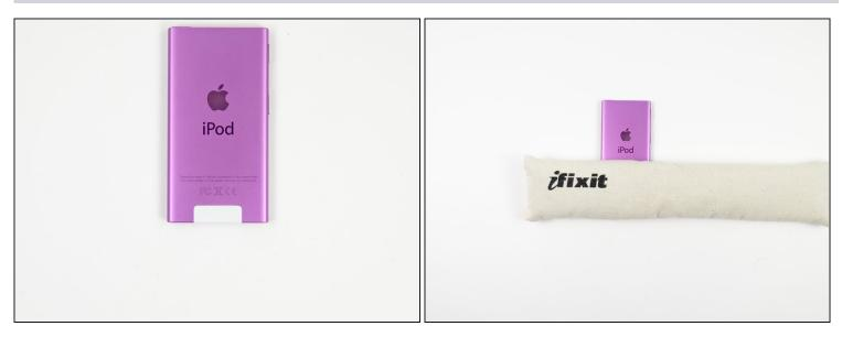
• Lay the iOpener over the plastic tab to loosen the adhesive. Let the bag sit on the device for approximately 90 seconds before attempting to open the panel.
