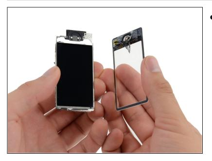
• Once all of the adhesive has been released, gently separate the display assembly from the front glass/digitizer.
