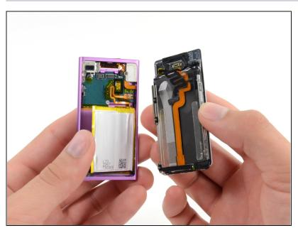
Completely separate the front panel assembly from the rest of the device.
