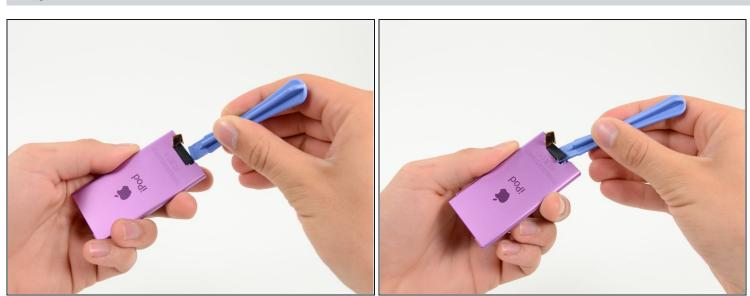
• Use a plastic opening tool to remove the black plastic spacer from the Nano.
