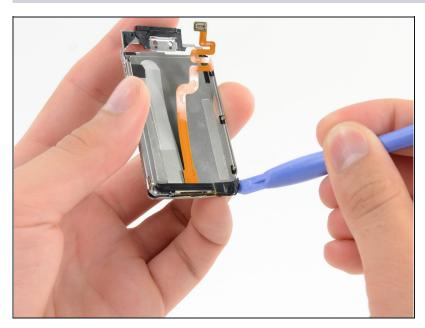
If there is tape holding the midframe to the display, remove it with a plastic opening tool.
