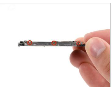
Remove the six (three on each side) 1.5 mm Phillips #000 screws securing the metal midframe to the display.
