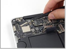
Use the flat end of a spudger to pry both antenna connectors up from their sockets on the AirPort/Bluetooth card, and move them out of the way of the card.
