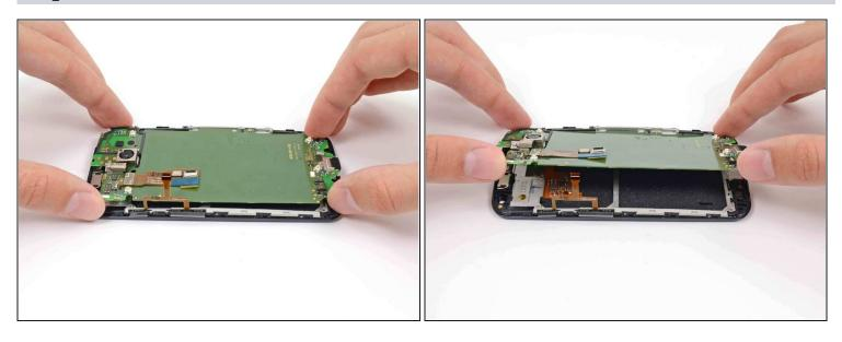
• Gently lift the motherboard out of the phone, rotating it from the SIM slot edge of the phone.
