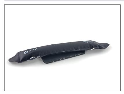
Heat an iOpener and lay it over the phone for approximately 90 seconds to loosen the adhesive securing the back cover.
