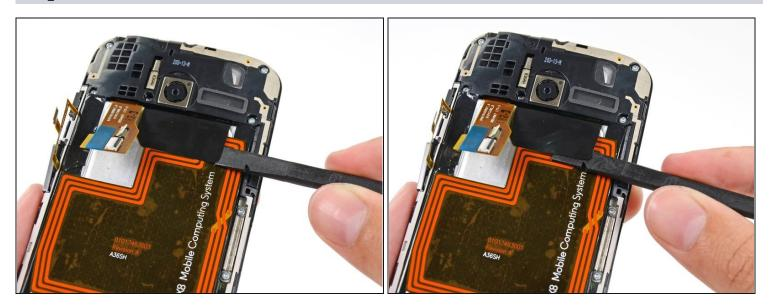
• Use the flat end of a spudger to peel the adhesive pull-tab off the top of battery.
