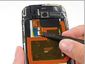
• Insert the flat end of a spudger under the interconnect cable to free it from the adhesive holding it to the battery.
