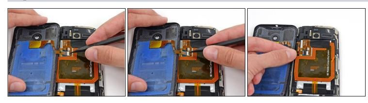
• Use the tip of a spudger to flip up the retaining flap on the flash cable ZIF connector.
