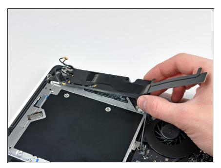
• Remove the rear speaker assembly from the upper case.
