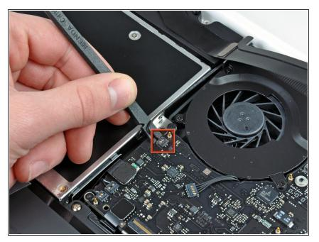
Use the flat end of a spudger to pry the rear speaker cable connector up off the logic board.
