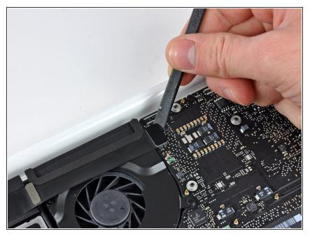
• Use the flat end of a spudger to pry the AirPort/Bluetooth cable connector up off the logic board.
