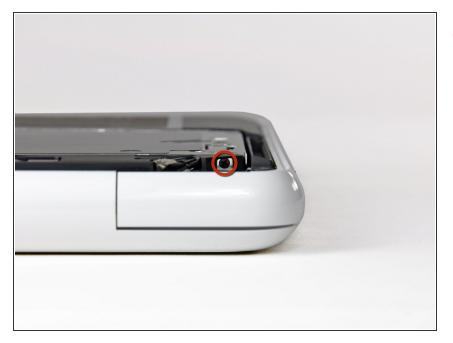
Remove the single 2.2 mm Phillips screw inserted horizontally into the side of the optical drive.
