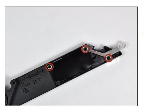
Remove three 3 mm Phillips screws securing the AirPort/Bluetooth board to the rear speaker assembly.
