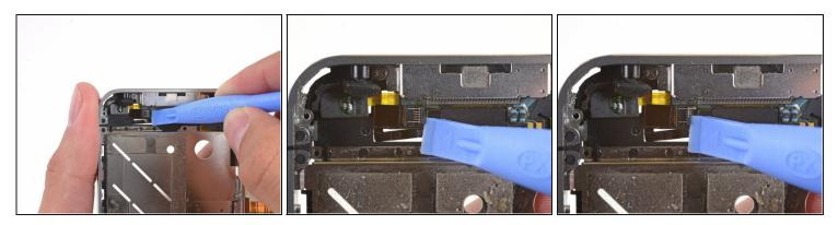
• Use the edge of an iPod opening tool or your fingernail to lift the home button ribbon cable retainer.
