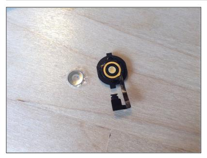
• You need really thin blade to carefully peel off the plastic film from the back of the button. Do NOT touch the glue with your finger!
