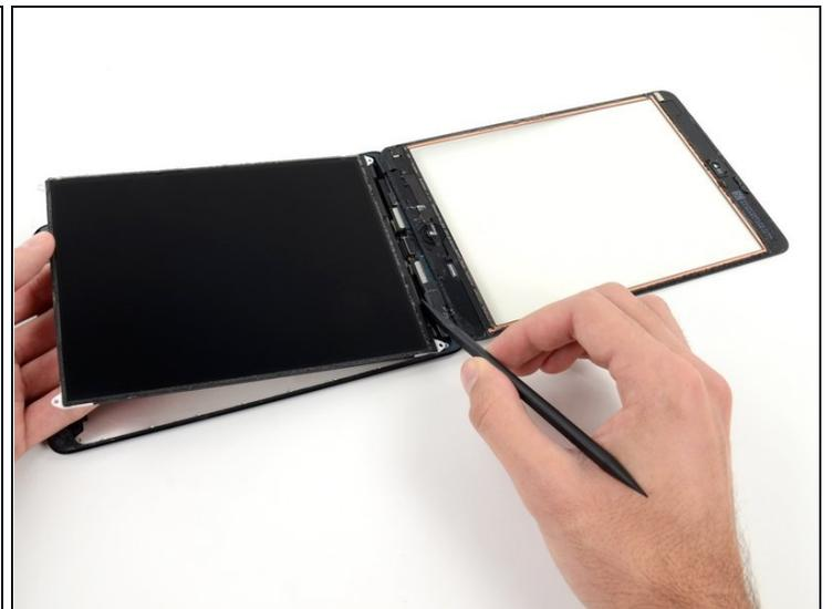
ⓘ Two wide strips of tape connect the LCD to the speakers.
