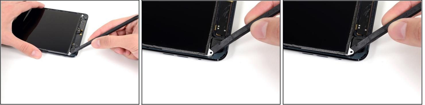
**i** In the next few steps, you'll be sliding a spudger between the LCD and the metal backing plate to fully separate the LCD from the adhesive beneath.
