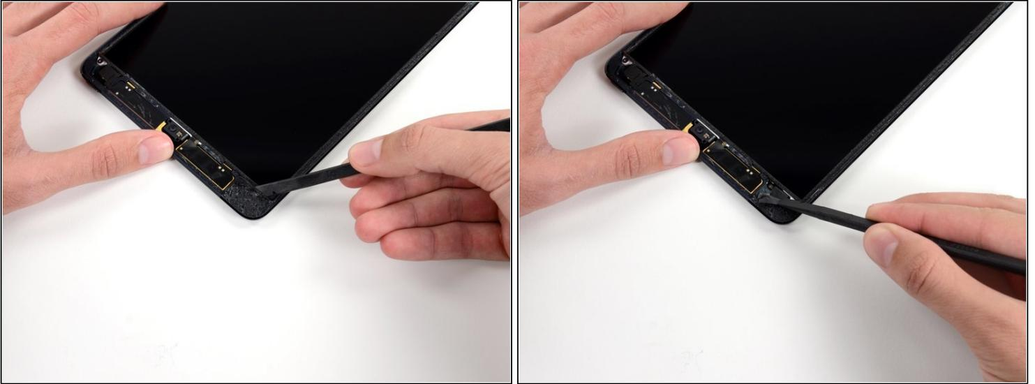
ⓘ The top left LCD screw may be covered by adhesive tape from the front panel.
