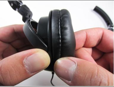
While holding the base of the ear cup with one hand, insert your index finger from your other hand into the inside of the foam ear piece.
