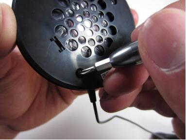
Remove the three screws located on the driver cover of the ear cup with the PH0 Phillips screw driver.
