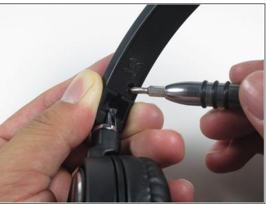
Remove the two screws on the underside of the headband with the PH0 Phillips screw driver.
