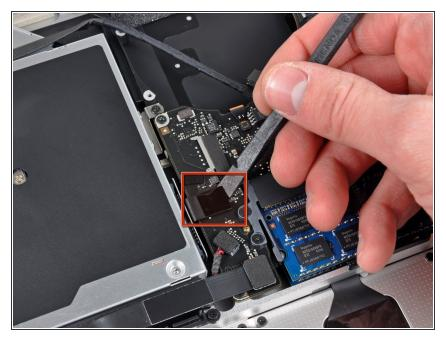
• Use the flat end of a spudger to pry the optical drive cable connector up off the logic board.
