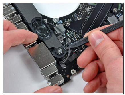
(i) If your microphone is still inserted into its void in the left speaker housing, use the tip of a spudger to lift it out.
