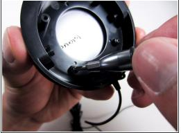
Remove the three screws located on the driver casing.
