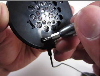
Remove the three screws located on the driver cover of the ear cup with the PH0 Phillips screw driver.
