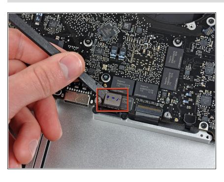
Use a spudger to pry the trackpad flex ribbon cable connector up off the logic board.
