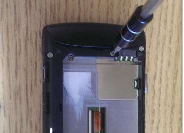
• Remove only the four screws circled in red using a Phillips #0 (PH0) screwdriver. Do not remove the others. The four circled screws hold the sliding screen down.
