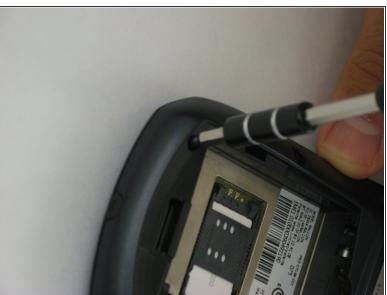
Use a T6 Torx screwdriver to remove the 6 screws holding the rear of the phone.
