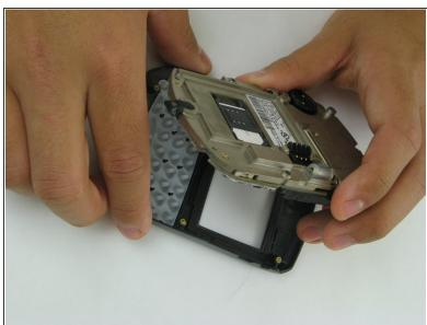
Pull the metal plate away from the front panel of the cell phone.
