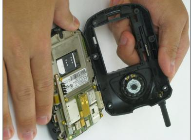
Slide the rear panel forward to reveal the motherboard.
