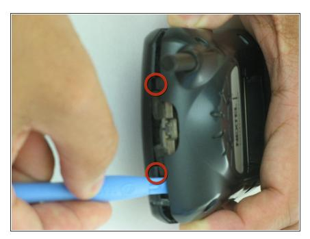
Repeat the process of unlatching the clips for the top section of the Blackberry.
