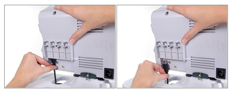
• Detach any accessory USB cables from USB ports on the monitor.
