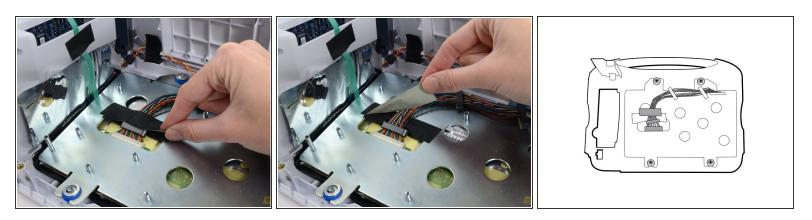
• Remove any tape from the LCD cable connector.
