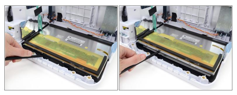
• Use the flat end of a spudger to lift the LCD out of the rubber gasket frame.
