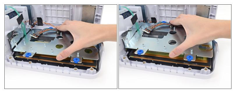
• Remove the LCD bracket.
