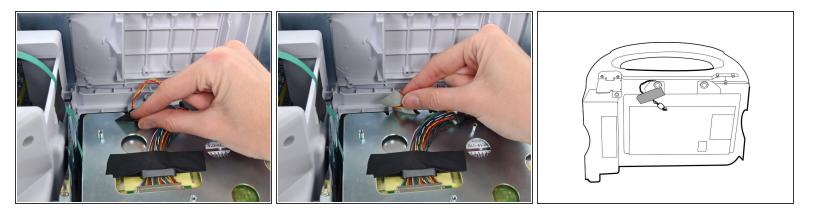
• Remove the light-bar cable from the LCD bracket and move it out of the way.
