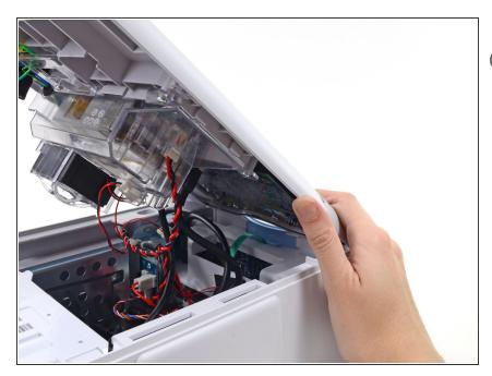
*i* Support the rear housing while you disconnect the cables in the following steps.
