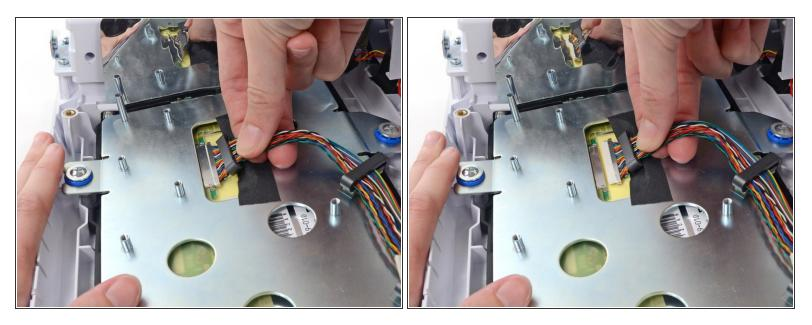
• Pull the LCD cable connector, firmly and evenly, straight out of its socket.
