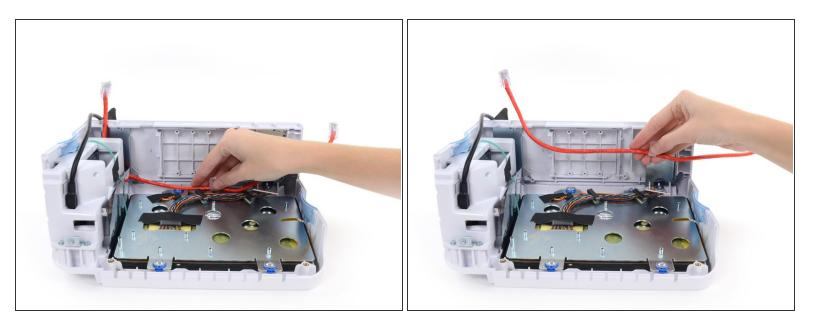
• Remove the ethernet cable, or simply tuck it out of the way.
