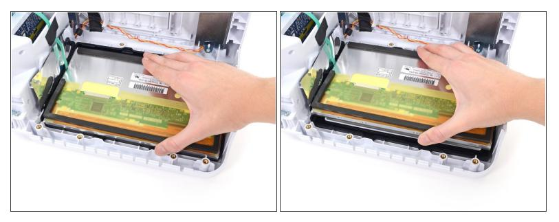
• Remove the LCD from the front housing.
