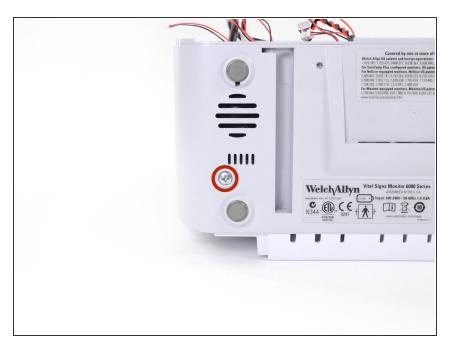
Remove the single Phillips #2 screw from the bottom housing near the speaker grille.
