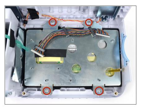
• Remove the four Phillips #2 screws from the LCD bracket.
