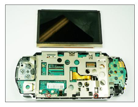
Now that the LCD is removed, unscrew the two screws in red.
