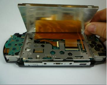
The LCD Screen is held by the LCD Frame with similar clips. Slide a thin tool between the clip and the screen and gently pry them apart while beginning to lift the screen.
