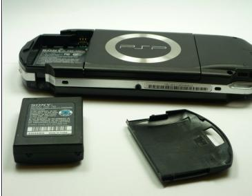
• Using your finger, remove the battery upwards from the system as shown.
