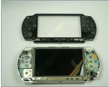
Gently separate the outer plastic casing from the rest of the system as shown.
