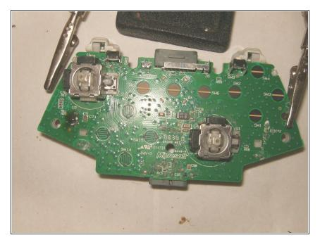
Here is the board with the new sticks and the left trigger button resoldered.
