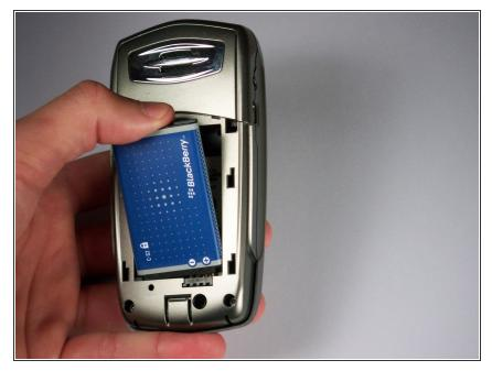
Remove the battery by pushing downward on the area where prongs connect to bottom inside of the phone while using a thumb, finger, or tool to pull on the top of the battery to lift it out.
