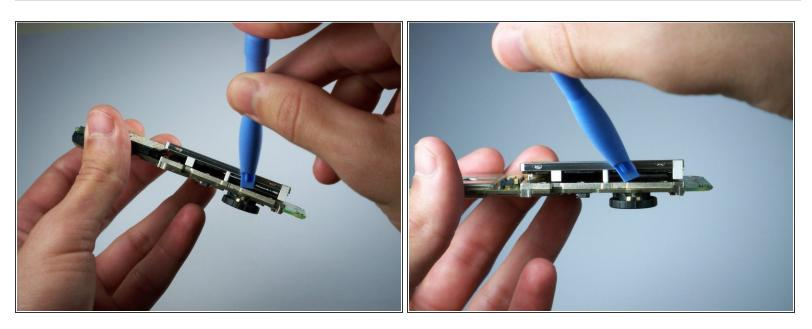
Wedge the BlackBerry opening tool between the adhesive and LCD, twist upward so the LCD becomes loose.
