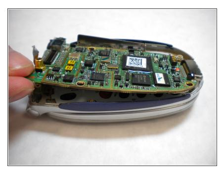
Gently lift a corner of the motherboard away from the casing to remove.
