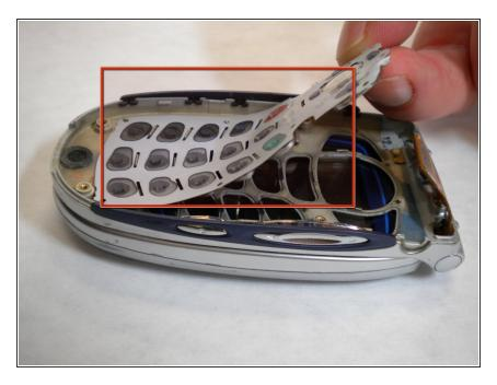
Peel the white keypad off the casing.
