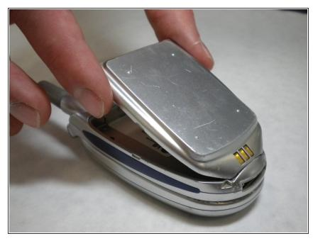
(i) Remove the battery by lifting up and rotating the battery away from the bottom edge.
