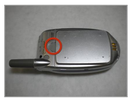
Locate the dark gray tab on the back of the phone towards the top. Push the tab towards the top of the phone to release the battery.
