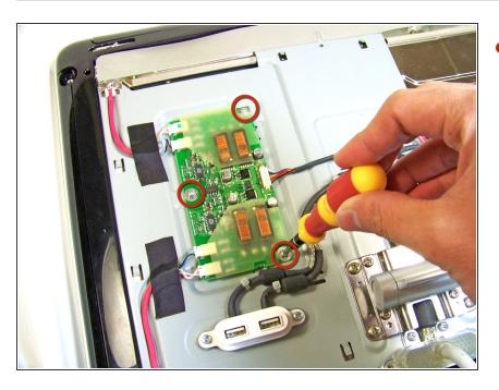
Remove these three screws holding the board to the display
