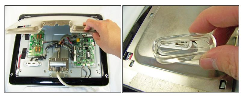
Now that the screw has been removed, slide the panel towards your body and lift it out.
