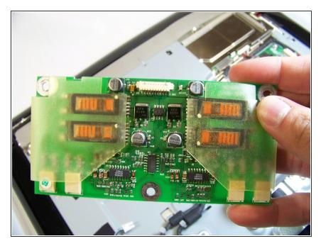
• Remove and replace the inverter
