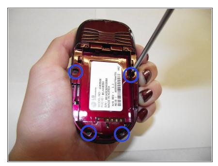
With a Phillips #00 Screwdriver, remove the four screws in a counterclockwise direction from the back cover. Set them aside on a surface where they won't roll away; these screws will be used in reassembly.
