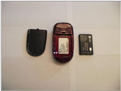
Place the plastic opening tool at the top of the battery and pry it out to remove. Set the battery aside.
