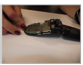
• When replacing the computer chip, the sensor bar for the volume button may pop out of place. If this occurs, gently push the bars back into place behind the buttons with your fingers.
