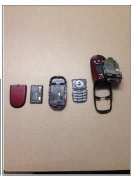
Remove the keypad using your fingers and set aside.
