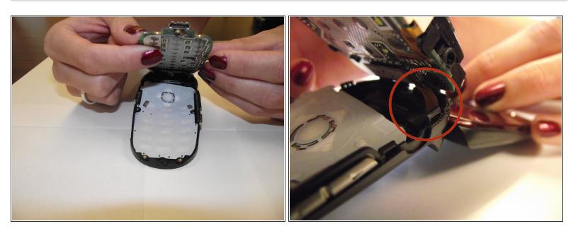
Gently lift the green computer chip plate out of the way to expose the keypad.
