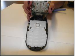
• Align the small holes in the new keypad with the posts on the phone.
