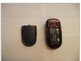
Using your thumb, slide battery cover off in a downward direction.
