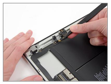
Use a pair of tweezers to peel back the adhesive tape covering the front-facing camera connector.
