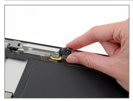
• Lift and remove the frontfacing camera from the iPad.
