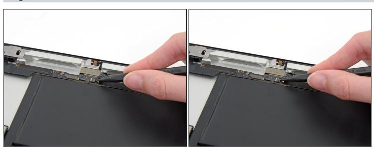
• Using the tip of the spudger, flip up the retaining flap on the microphone cable ZIF connector.
