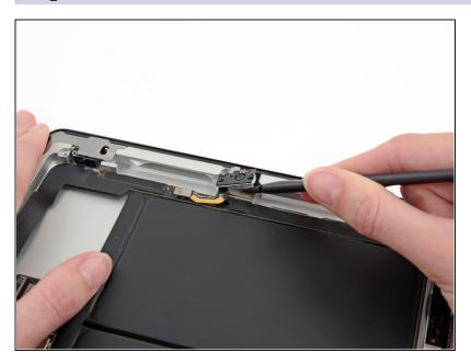
• Use the flat end of a spudger to pry the front-facing camera out of its recess in the rear case.
