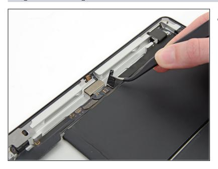
Use a pair of tweezers to peel back the adhesive tape covering the microphone ribbon cable.
