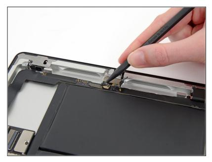
Insert the tip of the spudger underneath the microphone ribbon cable and carefully push it out from its socket on the ZIF connector.
