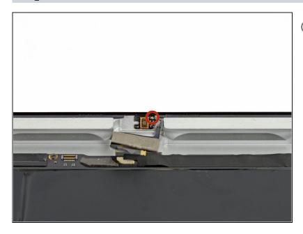
The next step will require you to pry the microphone assembly by using the small opening (highlighted in red) near the top right corner of the microphone assembly as leverage.
