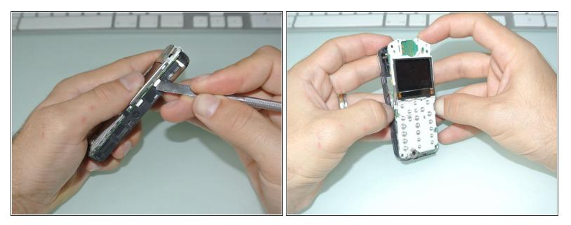
Use a metal spudger to pell off the four metal clips and separate the motherboard and keyboard from the main plastic part.
