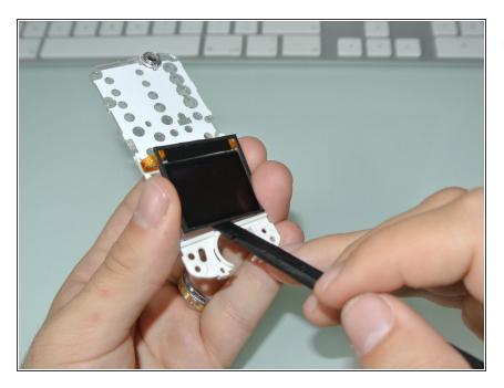
• Use a plastic spudger to release the disconnected screen.
