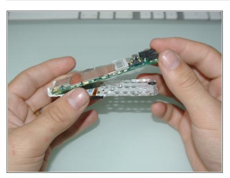
The last thing you need to doto access the Logic Board is to separate the Keyboard/Screen block just taking apart with your fingers.
