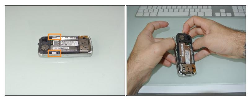
• You will see one plastic clip on each side of the device. Use your thumbs to push them apart and being able to separate the front case from the device other components.
