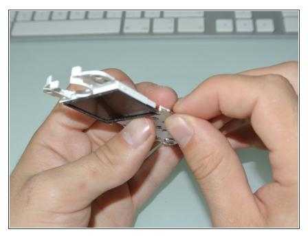
• Remove the two small metal clips keeping the cables safe.
