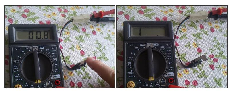
• check the conductivity with a multimeter. if the switch is faulty remove the green seal and drip some alcohol into the switch. Check the conductivity again. Let it dry upside down in a hot dry place. Buy a new one if it's still bad.
