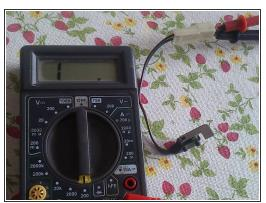
FIX: Disconnect power mains!!! remove the switch, check the conductivity with a multimeter. if the switch is faulty remove the green seal and drip some contact cleaner (alcohol) into the switch. Check the conductivity again. Let it dry upside down in a hot dry place.
