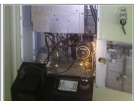
PROBLEM: faulty micro switch. FIX: Disconnect power mains!!! remove the switch, check the conductivity with a multimeter.
