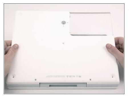
Once the front and sides of the lower case are free, turn the computer so that the back is facing you and pull the lower case up and toward you until the back tabs pop free (it may be helpful to jiggle the case up and down).
