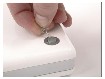
Use a pin (or anything you like) to remove the three rubber feet from the lower case.
