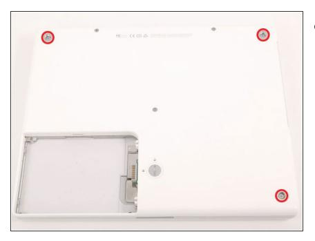
• Remove the three newly-revealed Phillips screws.
