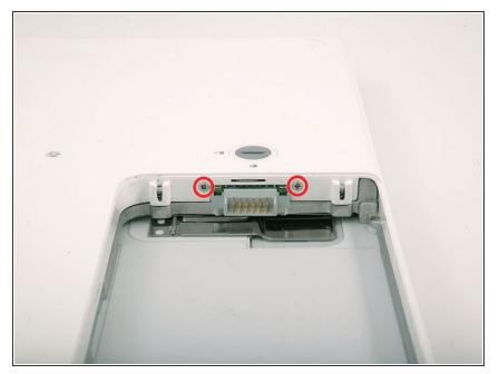
• Remove the two Phillips screws on either side of the battery contacts.
