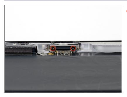
Remove the two 2.9 mm Phillips #00 screws securing the Lightning connector to the rear case.
