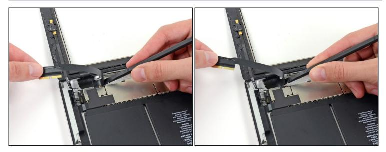
• Peel back the digitizer ribbon cable and use the flat end of a spudger to release the adhesive securing the cable to the rear aluminum case.
