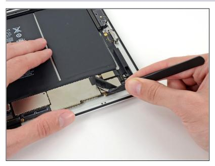
(i) If present, remove the piece of electrical tape covering the Lightning connector cable.
