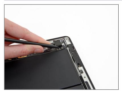
Flip up the retaining flap securing the volume/power button ribbon cable connector to the headphone jack assembly board.
