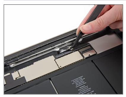
Use a pair of tweezers to peel back the piece of tape that secures the digitizer ribbon cable to the logic board.
