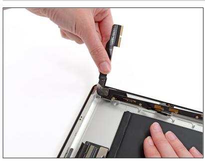
Holding onto the ribbon cable of the headphone jack assembly, carefully pull the assembly upwards towards the top of the device.
