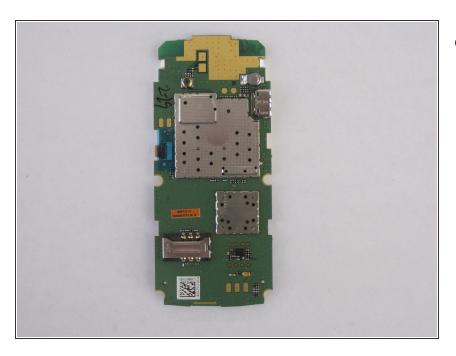
Place the circuit board with the display facing downward.
