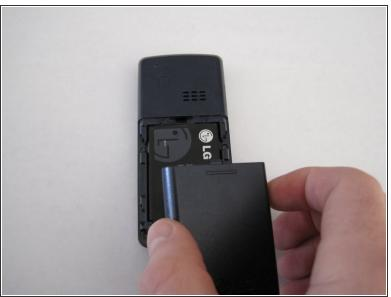
Slide the back cover down using your finger to remove the cover from the phone.
