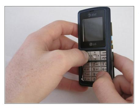
Push the contents of the phone away from the hardshell case by applying pressure to the keypad with both thumbs.
