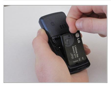
Press downward while pulling outward to remove the battery.
