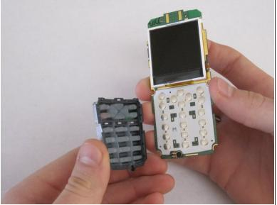
Separate keypad from circuit board by turning it upside down and allowing it to fall off.
