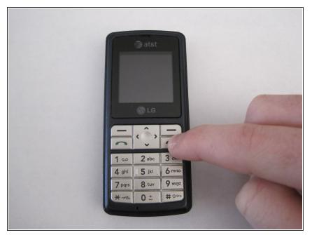
Power down the cell phone by pressing and holding down the red "end call" button.
