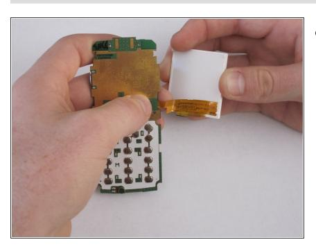
Carefully remove the electrical tape from the display.
