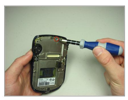
Unscrew to remove the back plate
