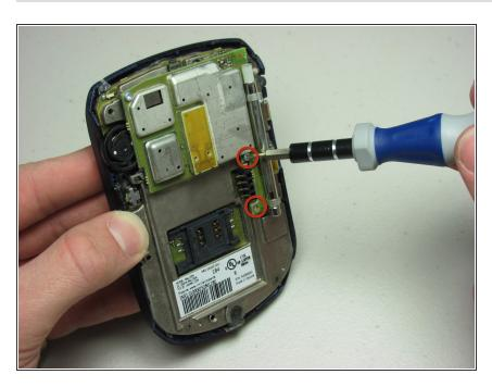
Unscrew the two screws with a T-6 screwdriver head
