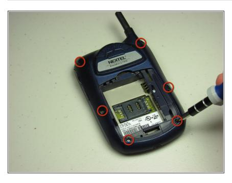
Remove the six screws with the screwdriver using the T-5 tip.
