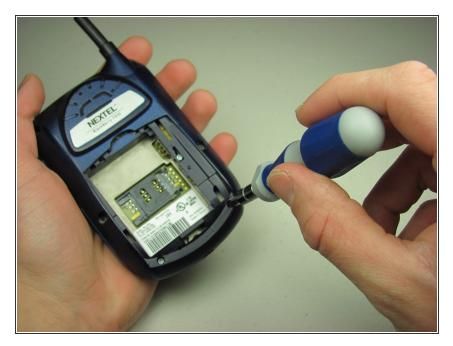
Remove the back cover exposing the battery, and remove the battery.
