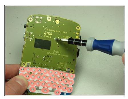
Using the Philips screwdriver unscrew center screw.
