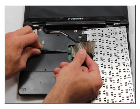
Wedge the spudger between the plastic clamp that holds the ribbon in place and carefully pry the connector off.
