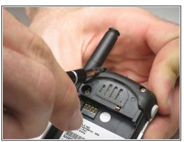
Using a small flat head screwdriver or your fingernail, remove the rubber covers near the top of the phone
