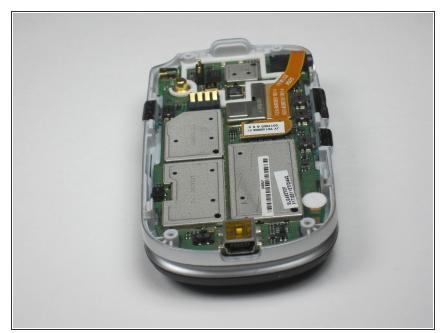
Make sure the phone appears as shown after removing the rear panel.
