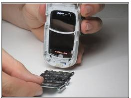
Gently remove the keypad from the phone by getting a grip on the top of the keypad and slowly peeling it top to bottom.
