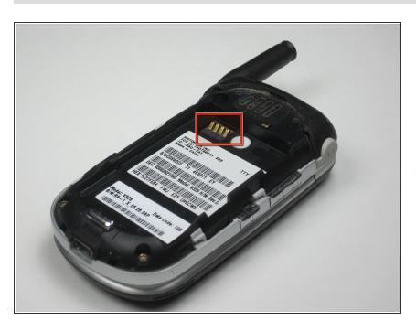
When replacing the battery, ensure that the side that has the "pull here" arrows goes toward the bottom of the phone. Place the side of the battery with the metallic contacts in toward the inside of the phone, making a full connection with the contacts within the phone (shown in the red rectangle).
