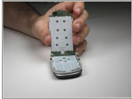
Gently lift up the logic board by placing your index finger at the top while keeping your thumb at the bottom of the phone for leverage.
