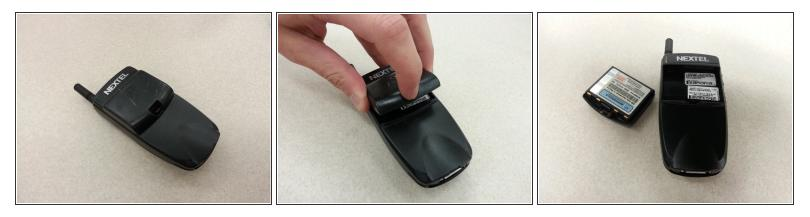
$\bigwedge$  Be sure phone is powered off before removing the battery.
