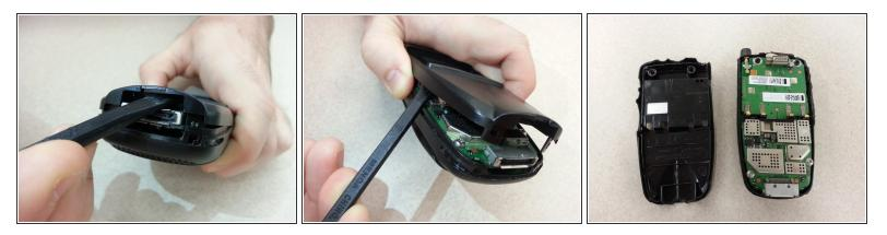
• Starting from the bottom and working towards the top, use a spudger to pry the back cover off the phone.
