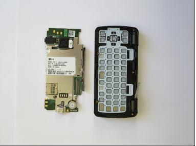
Using both of your hands, gently pry out the motherboard by pulling up on both ends.
