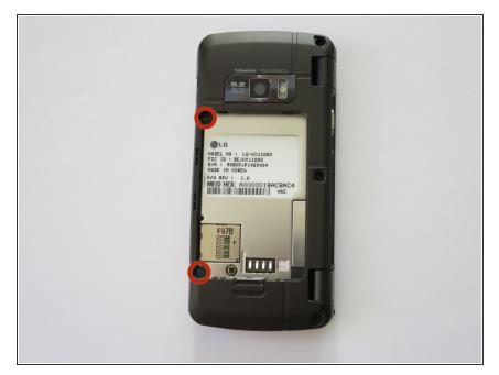
Locate the two inner 1.5mm #000 Phillips screws and remove them using a Phillips #000 screwdriver.
