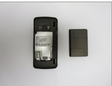
Lift the edge of the battery to remove it.
