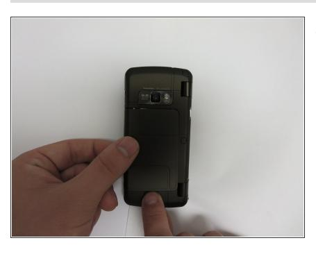
Slide the release latch down and toward you while lifting up on the left side of the battery cover.
